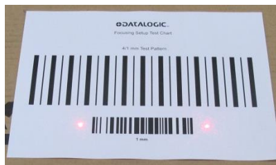
Figure 11 –Aligning the Focusing and PPI Setup Chart Using Laser Pointers as Reference
