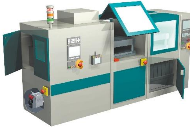
Fig. 4 Doors control by means of safety photocells
