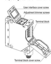
Tighten all screws surely to maintain the water-proof characteristics for IP67 (IEC/EN60529).
