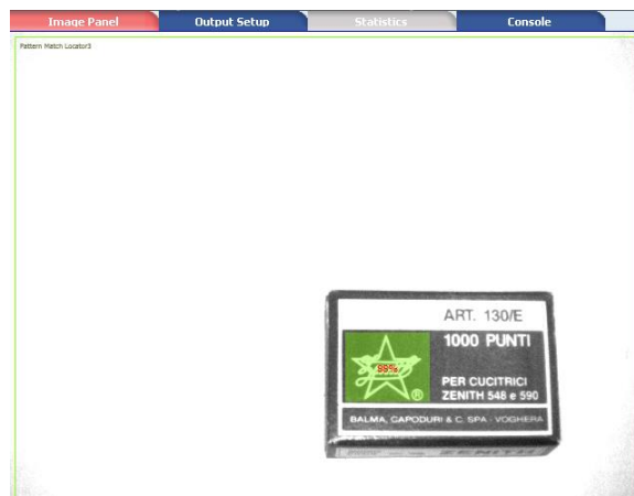
Fig. B Pattern Match Locator: Effect of a translated object
