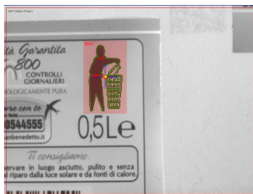
Fig. B 360° Defect Finder Control: Inspection effect on a faulty image
